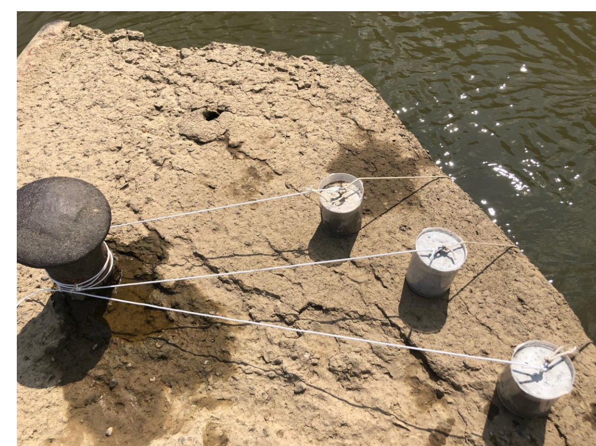
Figure 2. How substrates were fixed in the river
